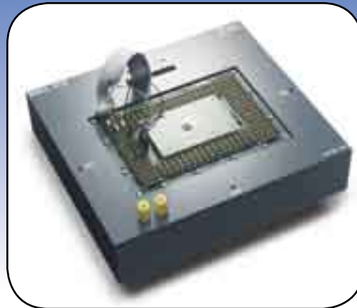
Fig. 4. Use of Outer Ring with the IC Adapter Board
