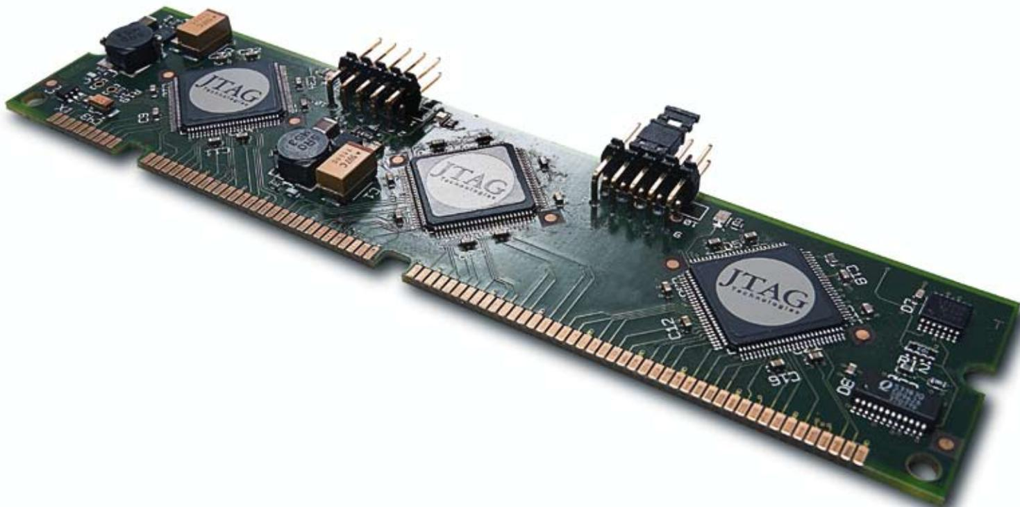
The JT 2128 is designed for easy insertion in standard 168-pin DIMM sockets either on a target board as illustrated above or in a test fixture. The five TAP-in and TAP-out signals (TDI, TDO, TMS, TCK, and TRST\*) are included among the 168 pins on the module connector and on two separate 10-pin connectors. TAP-in is the actual test access port for the module, and TAP-out can be used to daisy-chain to another DIOS module or to a scan chain on the target board.
